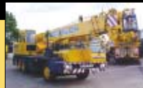
Tadano TL250E Year 1994/5. Capacity 25 tonnes. Truck Crane
