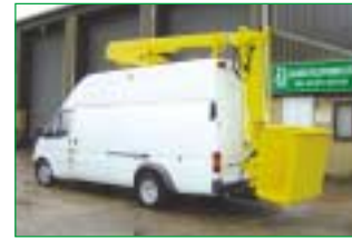
VEHICLE AND VAN 1997 VERSALIFT ET36NF 12.9m. working height (42ft.). Non HGV van mounted platform, re-painted.
