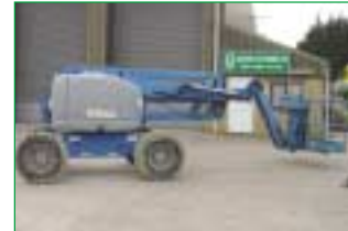
SELF PROPELLED TELESCOPIC 2001 GENIE Z45/25J 4X4 15.9m. working height (51.6ft) 4WD Rough terrain, Fly jib, Foam tyres
