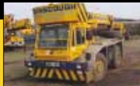
Grove, AP415 Year 1996. Capacity 15 tonne. Industrial crane
