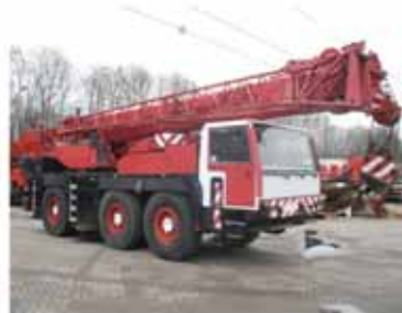
40 t, Liebherr LTM 1040-1, 1998
