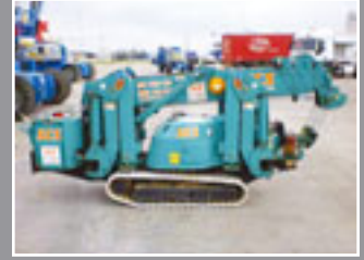
Maeda MC 285 CRM-E Mini-Kran 8,70m - 2,8Tonnen - 2006
