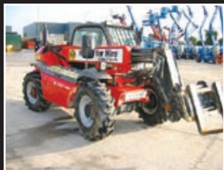
Manitou MLT523T Telestapler 5m/2,3Tonnen - 2006/7/8
