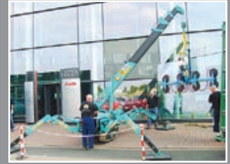
Maeda MC 285 CRM Mini-Kran 8,70m - 2,8Tonnen - 2006
