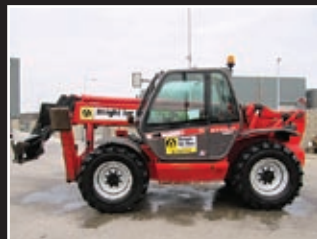
Manitou MT 1740 SLT Telestapler 17m/4Tonnen - 2005/6/7
