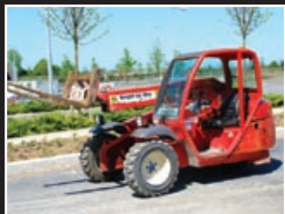
Manitou SLT415 Telestapler 4m/1,5Tonnen - 2003/4
