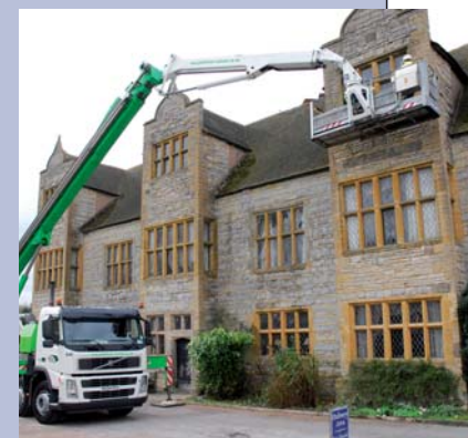
The Oil&Steel Eagle 44 was able to reach all access points from a single location.
