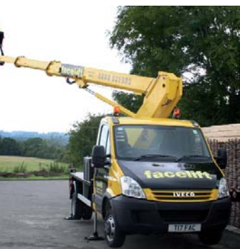
This is as far as the boom will rotate to the offside of the machine.
