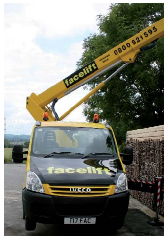
The Ascendant has vertical outriggers on the outside of the vehicle allowing it to set up in a single carriageway.
