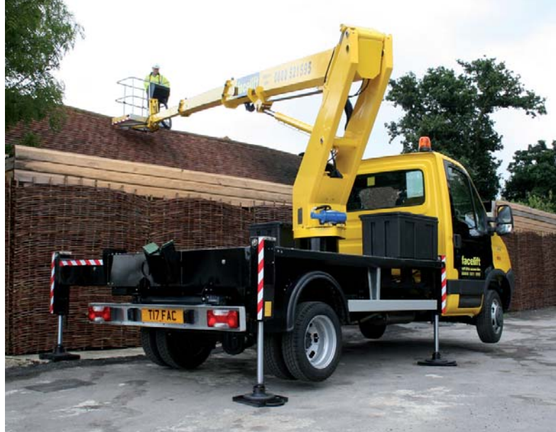
Mounted on a 3.5 tonne chassis, the Ascendant's 17 metre working height and basket capacity of 230kg, should be popular with new users.
