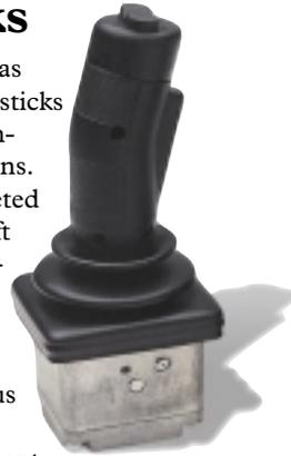
harsh environment. Mounted on a solid aluminium housing, several grip types can be mounted such as Ball grip, Rocker grip and/or Deadman grip. The joystick is based on contactless Hall-effect sensing and its lifetime exceeds 5 million cycles. Electronics are fully protected against moisture.
