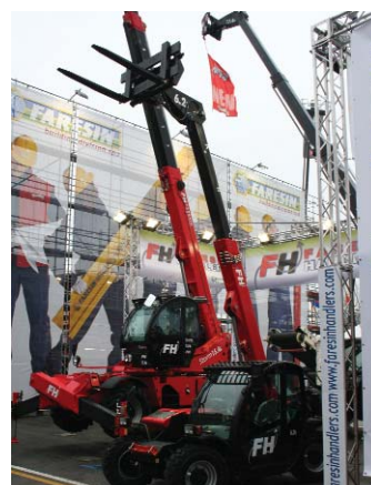
Faresin showed two new models - the 15.45 a 360 degree roto machine and the 6.25 compact model. Improved visibility to the right side of the machine is aided by a redesigned engine cover.
