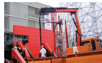
SAIE saw the culmination of four years of development work when Palfinger introduced its new 'High Performance' models with 80 variations being introduced over the next three. Features of the new machines include the new hexagonal boom, a 10 percent increase in capacity for a similar gross weight, a maintenance free boom system, more environmentally friendly corrosion protection and new control panel and hose protection. The launch acrobatics was pretty good too!
