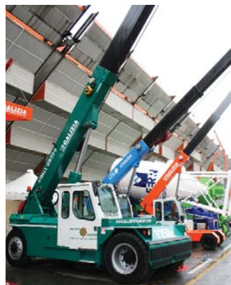
Italian manufacturer Galizia showed off several of its pick and carry cranes including its largest, the 25 tonne capacity F250E.
