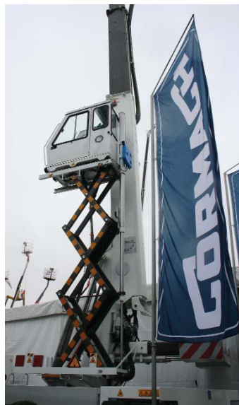
As well as its monster loader cranes, Cormach showed this elevating cab to help visibility when using the larger units.
