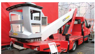
Originally unveiled at Bauma, SAIE was the first time anyone had seen Bison Palfinger's production version of its hi-spec TA25 Business truck platform mounted on a 3.5 tonne chassis.
