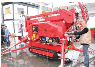
Italian manufacturer Tecchio showed three new platforms - two truck mounted and one spider. Biggest was the K427, a 27 metre working height, 7.5 tonne truck mounted platform with a jacking width of 3.2 metres and a working outreach of 13.4 metres. Mounted on a 3.5 tonne chassis, the 22 metre K422AT with an outreach of 11 metres, and the third new machine, the K622/DAT spider platform. Working height is 21.6 metres with 10.8 metres outreach. Width with the jacks out is 3.5 metres. The unit has a two tracking speeds up to 1.3 km per hour. All three lifts offer 265kg platform capacity.
