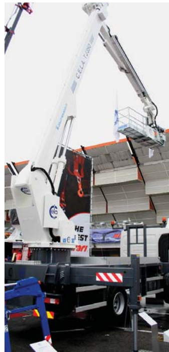
Cela showed its new T350, a 35 metre working height machine with up to 26 metres of outreach. Not many large Cela machines are seen in the UK but about eight fire fighting machines are now with the London Fire Brigade. Currently its biggest model is 54 metres although a 65 metre platform is scheduled for next year's SAIE.
