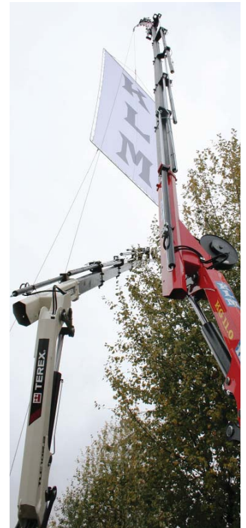
Italian loader crane manufacturer KLM has added a new model - the 11 tonne/metre KG11.0. Its products are also badged by Terex. KLM claims that it is the only manufacturer that has booms that extend past the vertical.
