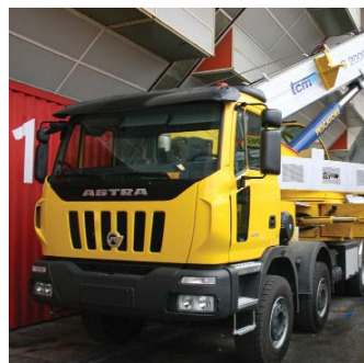
TCM showed its new C2000 - a compact 200 tonne crane mounted on a four axle Astra truck with an overall length of just 10.5 metres. The five section 28.8 metre main boom can also be equipped with an 11 metre, double extension jib.
