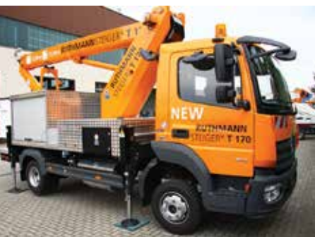
The new Ruthmann T170 is mounted on a 7.5 tonne chassis and has a 12 metre outreach.
