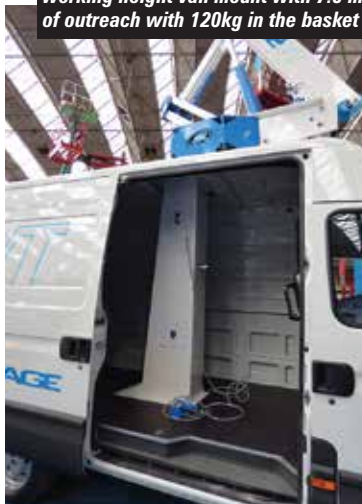
The Socage forSte 12VT is a 12 metre working height van mount with 7.5 metres of outreach with 120kg in the basket
