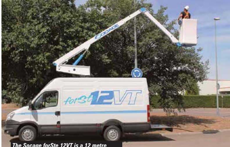
The Socage forSte 12VT is a 12 metre working height van mount with 7.5 metres of outreach with 120kg in the basket
