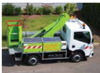
The France Elevateur Topy has 11 metres working height and can carry up to 500kg. This is the electric eco version with solar panels to help recharge the battery.
