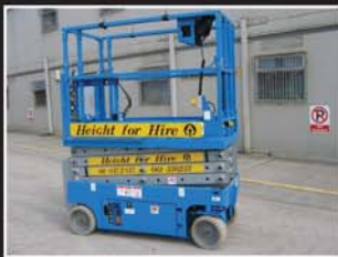
Genie GS1932 battery scissors 7.6m - 2004/5/6/7
