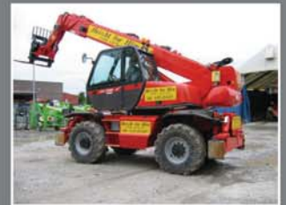
Manitou MRT2150 diesel teleporter 21m/5tonnes- 2005
