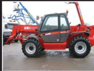
Manitou MT1335 diesel teleporter 13m/3.5tonnes – 2005
