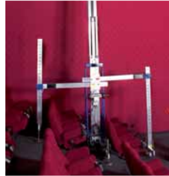
The Böcker Alp-Lift range includes the Kinolift PHC1000S which can straddle rows of seat and deal with slopes
