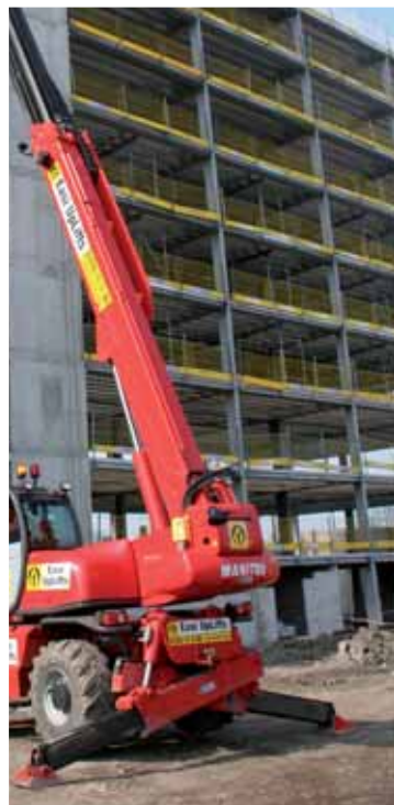
One of the Manitou MRT 2540 telehandlers placing materials on the upper floor.
