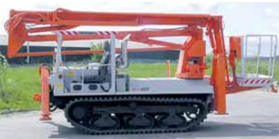
An earlier Marooka platform, a Pegasus, mounted on the company's MST 600V chassis.
