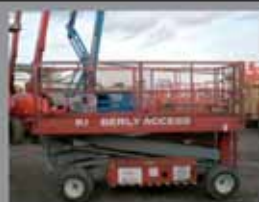
Upright SL26 Diesel Scissor 10M working height
