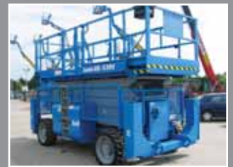
Genie GS-5390 RT Diesel Scissor 18.5m - 2005/6/7
