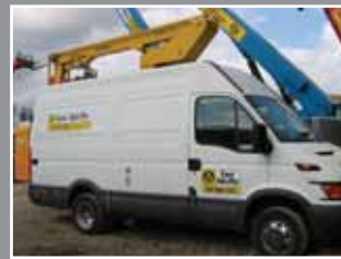
GSR 12.5RA (Iveco) Vehicle-Mounted 12.5m - 2003
