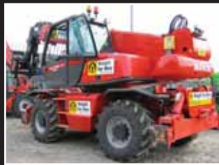
Manitou MT 2150 Telescopic Forklift 21.0m/5.0 ton - 2004/5
