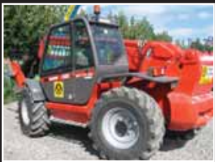
Manitou MT 1740 Telescopic Forklift 17.0m/4.0 ton - 2005
