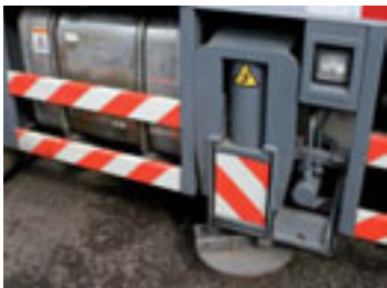
Aluminium fuel tank and outrigger lighting are recent Zoomlion additions.
