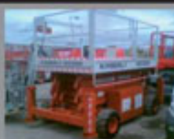
Snorkel 4084 Diesel Single Deck Extension Scissor 4 wheel drive jack legs 14M working height
