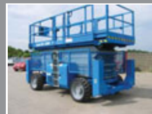
Genie GS5390 Diesel scissors 18.5m - 2005/6/7
