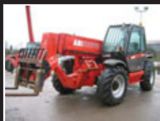
Manitou MT1335 Diesel teleporter 13m/3.5 tons 2005
