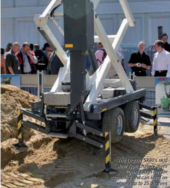
*The Leguan SX80's skid steer type chassis gives good rough terrain capability and can level on slopes up to 25 degrees.*
