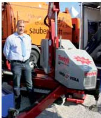
of 2.9 metres long from the centre of the machine. Using a lightweight Amco Veba crane, it has a maximum capacity of 1.75 tonnes and can lift 290kg at 10.9 metres. Standard equipment includes a built-in generator, wireless remote control and GPS/GSM for remote trouble shooting and information access.
