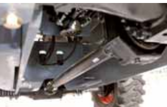
The unusual drive train is based on telehandler axles.
