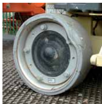
JLG's welded steel wheels were too easily damaged.
