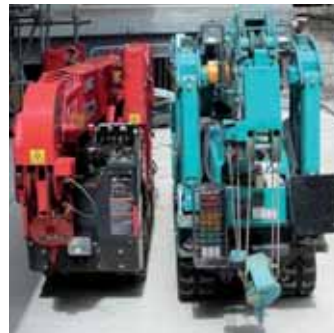
Despite very similar performance, the Maeda MC285 is significantly wider than the Unic 295.
