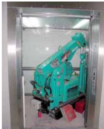
For their lifting capacities, spider cranes are incredibly compact.
