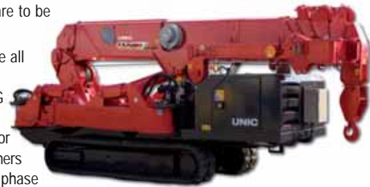
The Unic URW-706 is the largest spider crane from any manufacturer to date.
