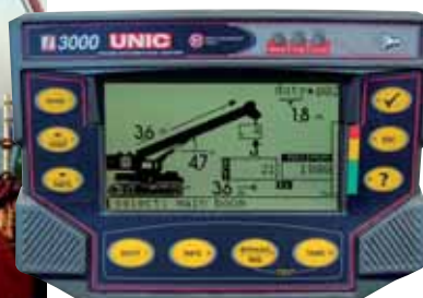
Full safe load indicator on a Unic 376 and 506.
