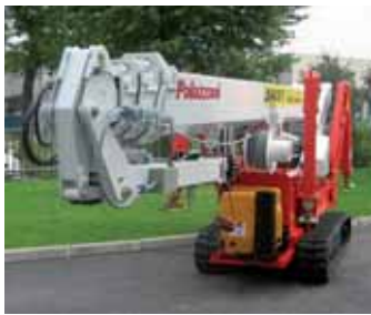
The Palazzani XTJ30 (above) and the XTJ35 have 600kg winch options and can lift to 30 metres.
