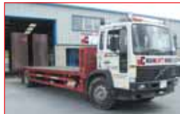
00 VOLVO FLC 18 Complete with 3DF beaver tail body and remote control winch
