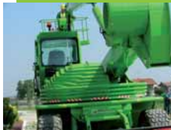
The counterweight is raised as the lower boom goes up
