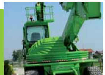
The counterweight is raised as the lower boom goes up
