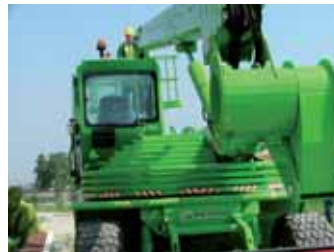
The counterweight is raised as the lower boom goes up
