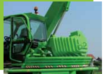
The counterweight is raised as the lower boom goes up
