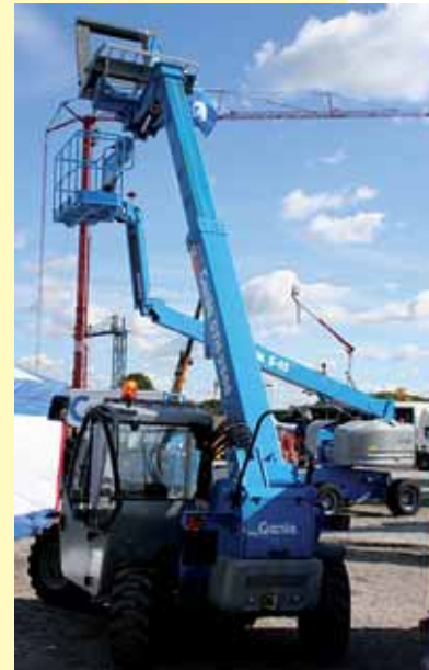
Genie showed its latest telehandler - the compact GTH 2506 with six metre lift height and 2,500kg lift capacity - along with a good selection from its aerial lift line.
