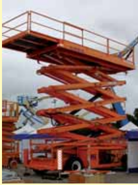
The worlds largest self propelled scissor lift, the Holland Lift G320 with 34 metre working height towered over most of the exhibits. Russon Access also showed a range of models from the Manitou line up.
