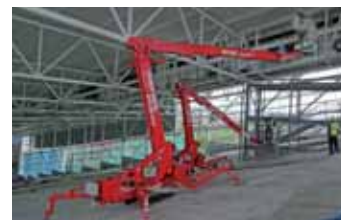
The Teupens were equipped with special wedge shaped outrigger mats.
