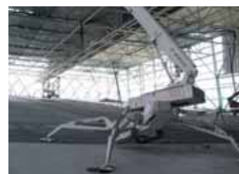
The Ommes were able to handle the 15° slope but used the non slip mats.
