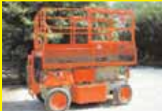
JLG 3969-E (1999) Self propelled scissor lift. 45' working height. Battery. Repainted, serviced & tested.
