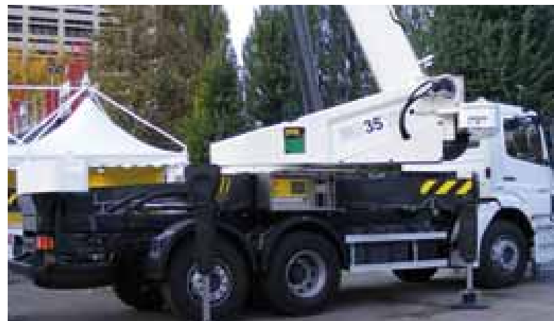
Fiorenzo Flisi who acquired Mister Gru, has re-jigged the crane range and introduced the new MG35TK which uses the same boom as the MG35HS and is mounted on a 26 tonne truck chassis.
