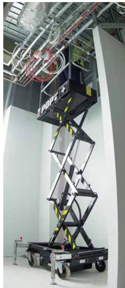
The Pop-Up+ has a work height of up to 4.5 metres.
