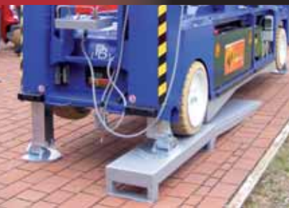
PB offers levelling jacks on all of its narrow scissors which now range to 20m high on a 1.2m chassis.
