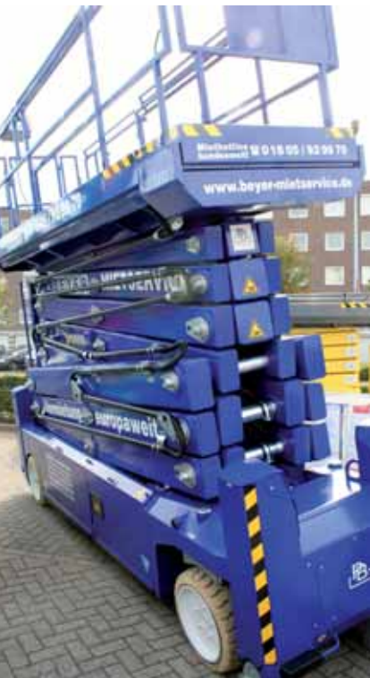
PB offers levelling jacks on all of its narrow scissors which now range to 20m high on a 1.2m chassis.
