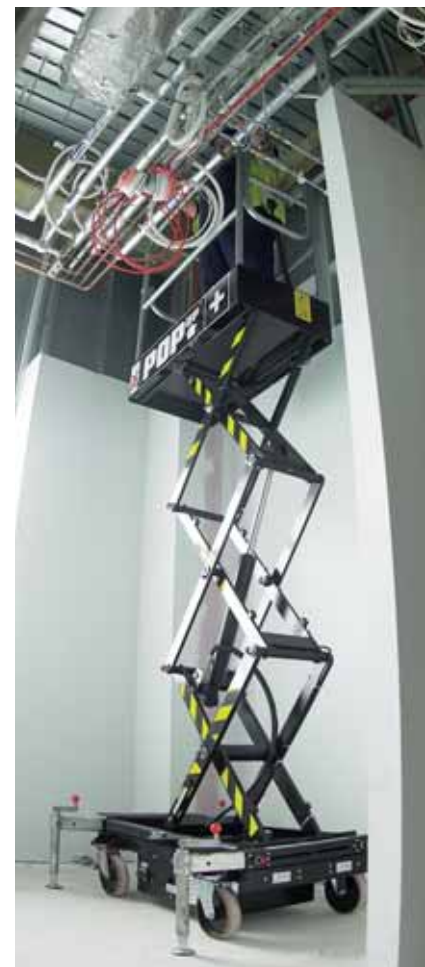
The Pop-Up+ has a work height of up to 4.5 metres.
