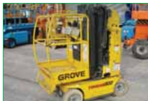
PERSONNEL PLATFORM 2000 Toucan 800 8m working height (26ft) Compact Design
