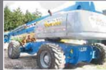
Genie S125 Telescopic diesel boom - 40.1m 2003/4/5/6/7
