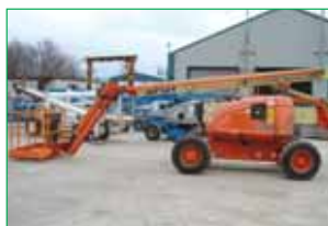
SELF PROPELLED TELESCOPIC 1999 JLG 600AJ 20m. working height (66ft). Articulated Jib.
