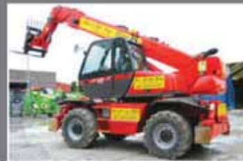
Manitou MRT2150 Rotator teleporter 21m/5T - 2005
