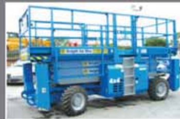
Genie GS5390 Diesel scissors 18.5m 2005/6/7
