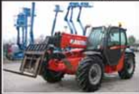
Manitou MT 1030 Telescopic Forklift 10m/3 ton - 2005
