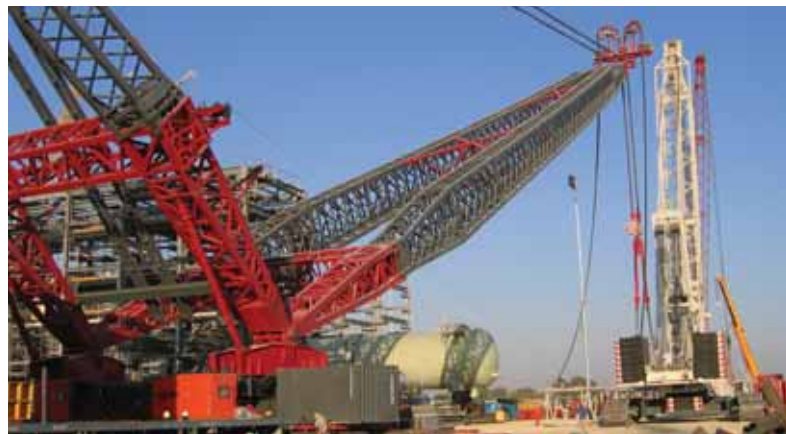
The ALE SK90 completes its first commercial lift - 755 tonnes at 84 metres.
