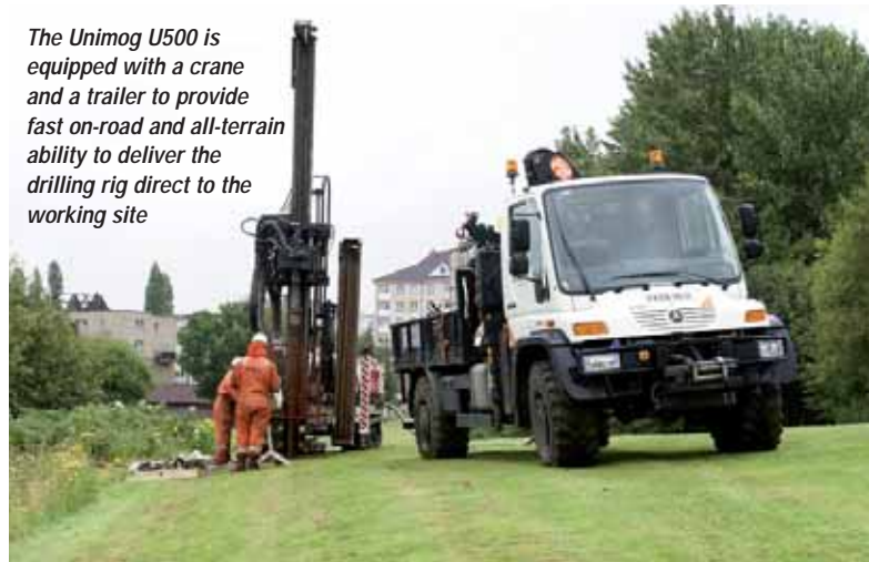
United Utilities uses this unit with 16t/m crane to deliver and place poles in remote locations
