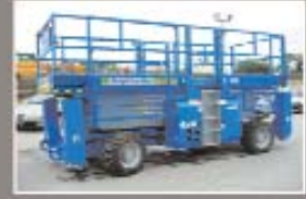
Genie GS-5390 Diesel Scissor 18.5m
