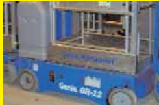
GENIE RUNABOUT GR12 (2002) Self propelled personnel lift. 18' working height. Battery. Serviced & tested.
