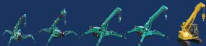
MC104 Lifting Capacity 995kg x 1.1m MC285 Lifting Capacity 2,82t x 1.4m MC305 Lifting Capacity 2,98t x 2.5m MC405 Lifting Capacity 3,83t x 2.7m LC785 Lifting Capacity 4,9t x 2.1m
