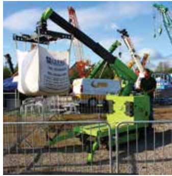
Hook-Up Solutions' new 1.5 tonne Hooka pick&carry crane with 700mm longer boom to lift pallets or bulk materials bags.
