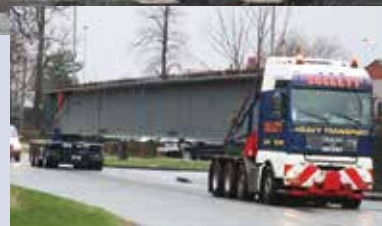
The Doll Bogie is ideal for transporting long, heavy loads, such as steel bridge beams.
