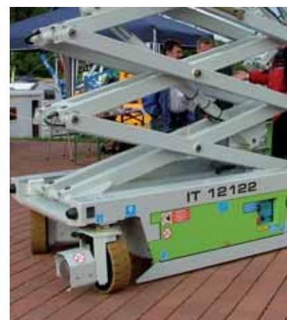
Iteco quickly adopted UpRight's over-centre steering design and more recently followed JLG with direct electric drive.
