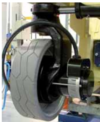
JLG introduced the first direct electric drive on its ES series scissors in 2003.
