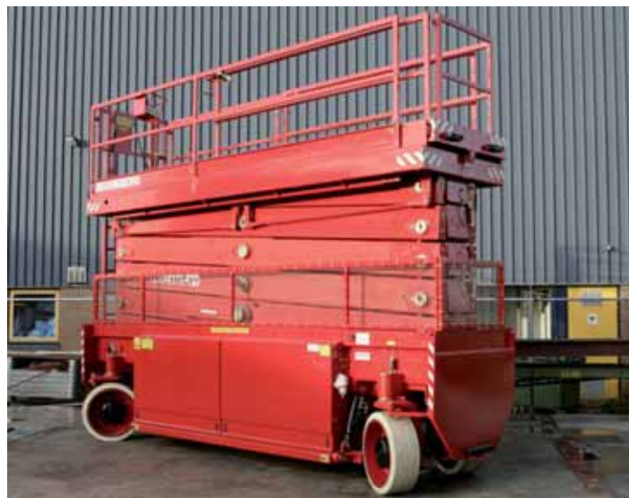
The largest electric scissor lifts from Holland Lift are now being equipped with four wheel drive and four wheel steer in order to provide better manoeuvrability.
