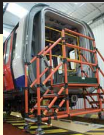
Planet Platforms supplied 13 GRP steps to Bombardier Transportation where they are used to test the new carriages at one of the facilities in Derby
