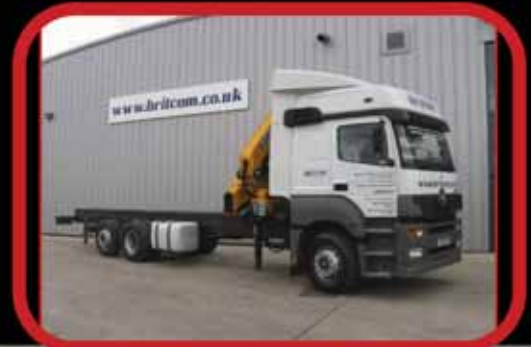
Mercedes Benz Axor 2543 2004 (54). 6x2 Rear Lift. Fitted With New Effer 340-4S (4 Extensions) with Radio Control. Rear Stabilisers. 26,000kg GVW. 44,000kg GTW. Air & Electrics For Drawbar Use.
