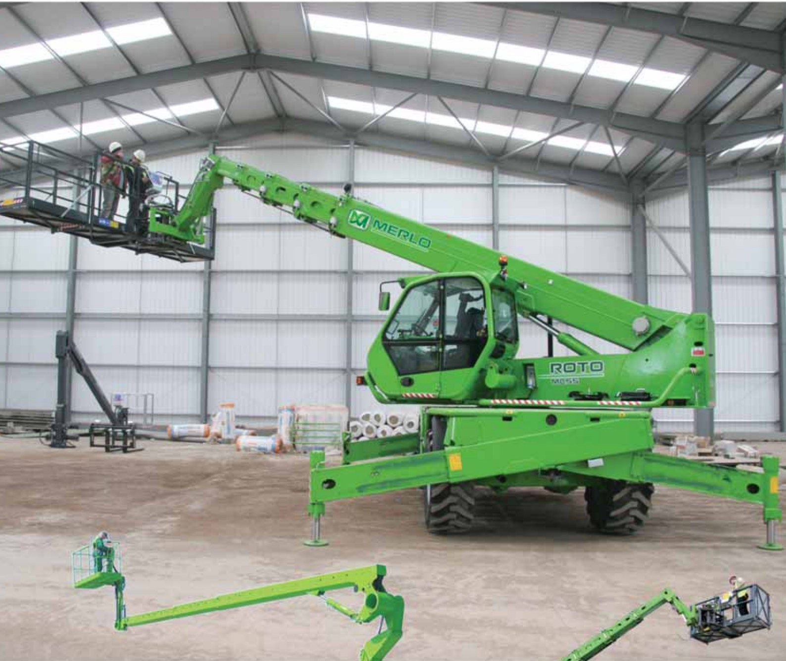
MRP Operating heights 20m - 30m Travel speed up to 40 km/h in cab. Travel on-site at up to 5 km/h
