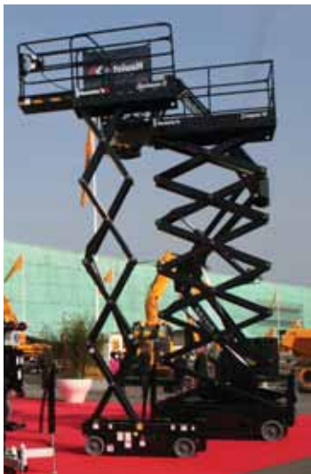
Haulotte unveiled the Compact 14 - a 12 metre platform height, 1.2 metre wide scissor lift
