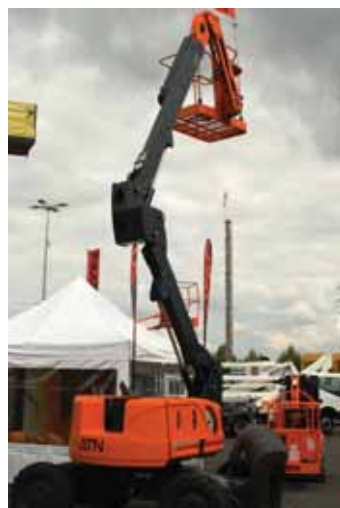
ATN's first boom lift - the 12 metre rough terrain Zebra 12 has its own built-in diagnostic screen.
