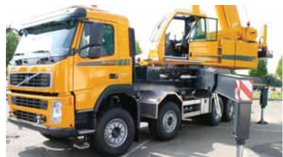
The Marchetti MTK 1006 mounted on a four axle Volvo FM 84R truck chassis has a lift capacity of 80 tonnes and max tip height of 55 metres with jib.
