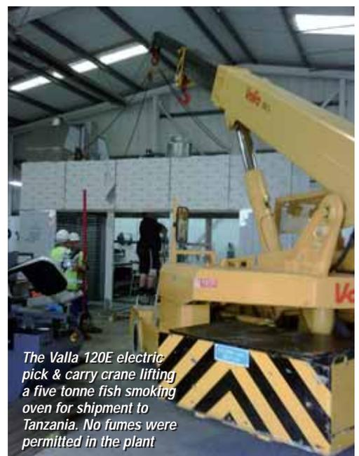
*The Valla 120E electric pick & carry crane lifting a five tonne fish smoking oven for shipment to Tanzania. No fumes were permitted in the plant*
