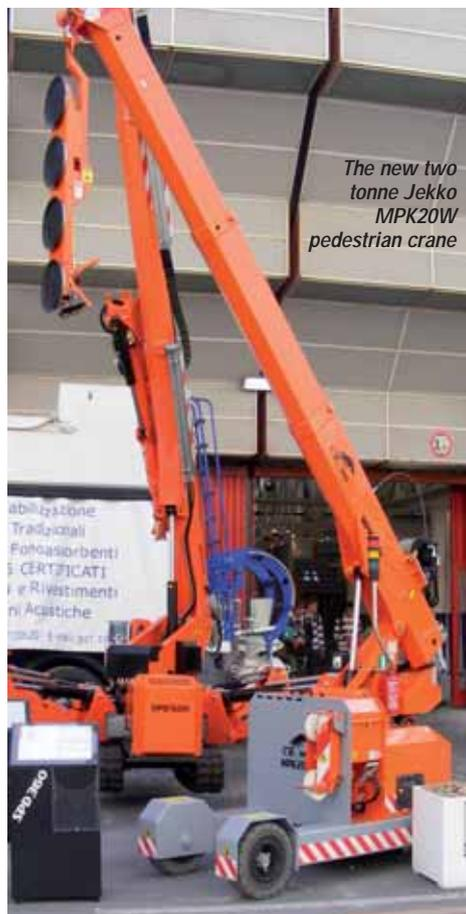
The new two tonne Jekko MPK20W pedestrian crane
