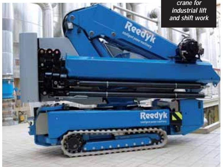
capability. With rubber track shoes and the ability to get in close they can offer a good solution for smaller moves.
