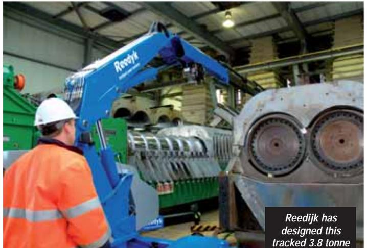
Reedijk has designed this tracked 3.8 tonne crane for industrial lift and shift work
