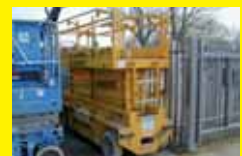
LIFTLUX SL105-10 (2002) Self propelled scissor lift. 41' working height. Battery. Repainted, serviced & tested.
