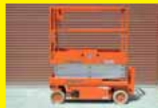
SNORKEL S1930 (2006) Self propelled scissor lift. 25' working height. Battery. Serviced & tested.
