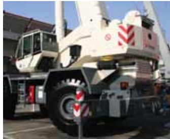
The Terex RT100 features a 53.1 metre, six section boom with a maximum tip height of 55.8 metres.
