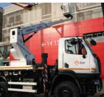
The Scorpion 15E is a 17 metre working height, straight boomed platform mounted on an extended wheelbase Mercedes Unimog U20.
