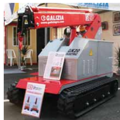
The Galizia GK20 is an all electric, two tonne capacity pick and carry crane.
