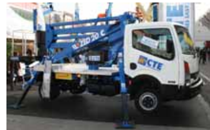
The new CTE Zed 20C has 20 metres working height and 9.2 metres outreach.
