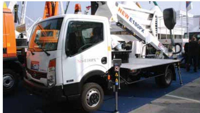
One of three new truck mounted platforms on the GSR stand - the 18 metre E180PX
