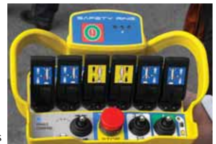
A three stage LED panel alerts the operator to the status of the Safety Ring, so that he is aware if a controller shut down is due to the Safety Ring or another issue.
