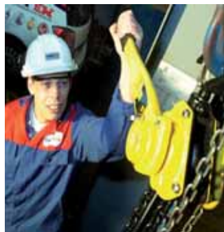
To prevent damage when using chain blocks, use an overload protection system such as Load Safe.
