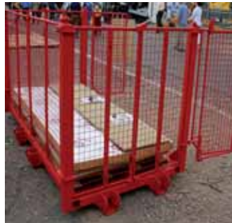
This novel sheet/materials handler (for crane or telehandler) was spotted on the Nethergate Developments stand.
