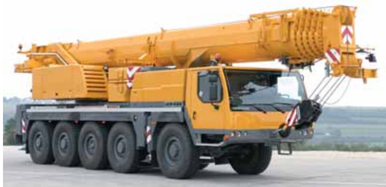
The LTM 1095-5.1, launched just over two years ago, has a 100 tonne nominal rating in spite of its name.
