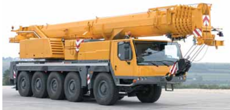
The LTM 1095-5.1, launched just over two years ago, has a 100 tonne nominal rating in spite of its name.
