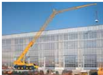
Liebherr currently has four mobile cranes that it considers to be in or around the 100 tonne sector. This is the LTM 1100 4.1
