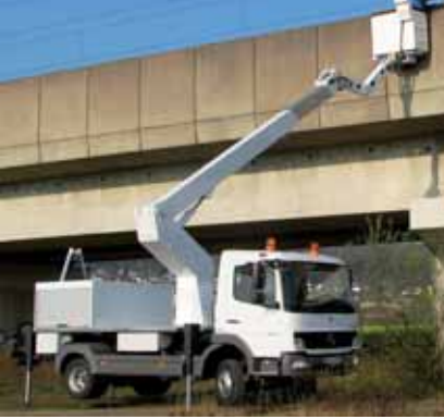
Mounted on a Merc 7.5 tonne chassis, the Esda TG1800 has an 18 metre working height narrow operational width.
