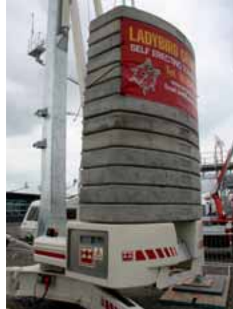
The CBR 32 Plus now features the controls within the ballast. Look out for the CBR26 Plus in July.
