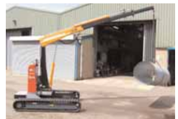
The TP2000/FV1200 can handle 250kg at 4.3m and with the boom stowed it measures 1.9m x 1.74m and 2m high
