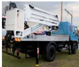
The 25 metre, 10kVa insulated unit was unveiled at Vertical Days in June. Mounted on a 14 tonne chassis it has been designed specifically for the harsh Middle East climatic and operating conditions.
