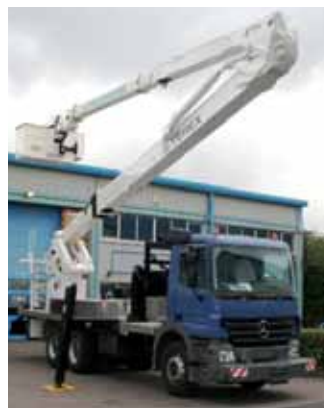
The platform is mounted on an extended Mercedes Actros 3340 chassis and has a 360kg capacity two man basket, a 680kg lift capacity jib and full insulation to 69kVA.
