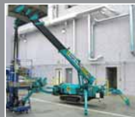
MAEDA MC 285 CRM Mobile minicrane 8.7m/2.8 Tonne - 2006
