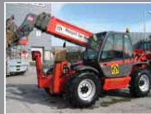
Manitou MT 1740 Telescopic forklift 17m/4 Tonne
