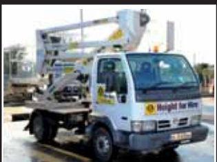
GSR 198PX Van mounted on Nissan Cabstar 19.50m - 2005
